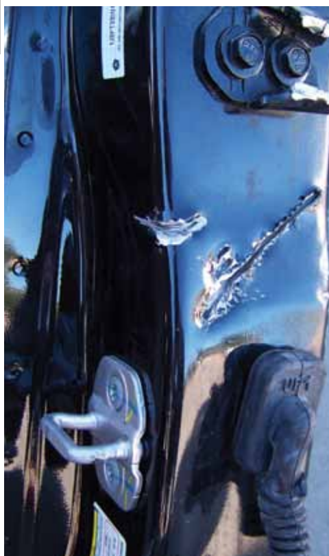
After repeated unsuccessful attempts to cut into or through a Boron B-pillar with various air chisels, the tests were stopped. The chisel was only able to cut into the outer mild steel layer and would not cut through the inner Boron.
