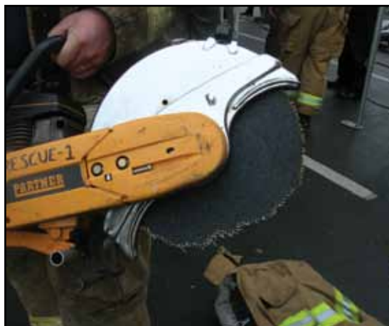
Cutting through the hardened advanced steel of the B-pillar destroyed the abrasive blade of the rotary saw. As expected, significant showers of sparks were generated during use of the saw, making this an unrealistic tool for extrication operations.
